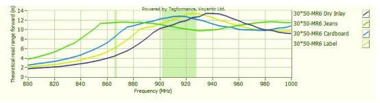
Sensitivity&Read Range Test power: 4W EIRP
